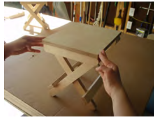
Align stool and check to make sure everything is pressed together and the glue held.
