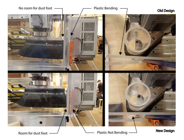
This image shows a comparison of the dust foot interacting with the mini enclosure at the limits of the machine travel. Note the flexing of the plastic of the mini enclosure in the top part of the image. The bottom part of the image shows the revised design of the enclosure, which eliminates the stress on the enclosure.
