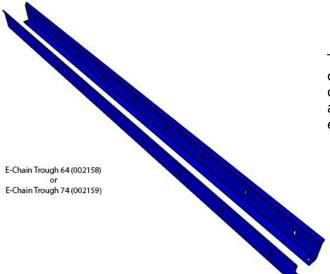
The E-chain trough will support the chain when traveling down the length of the tool. The E-chain trough also acts as an anchor point for the lower end of the E-chain.
