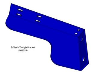
The E-chain trough bracket mounts to the underside of the table side extrusion and rests on the side of the table leg. It serves as a mounting point for the trough.
