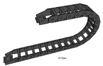
The E-chain will come sized to match the length of ShopBot's X-axis that it was ordered for. It is designed to be center-mounted, meaning that it will be shorter than the actual length of the machine.
