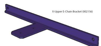
This bracket mounts to the outer side of the gantry end plate and serves as an attachment point for one end of the chain.
