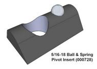
One of the specialized pieces of mounting hardware is the Ball & Spring Pivot Insert (000728). Two of these will be used to mount the E-chain trough brackets to the underside of the table extrusion. Their function is to slip into the slot of the table extrusion and rotate into position before being tightened.
