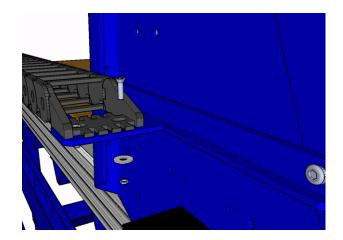
Secure E-chain to trough with flat head screws, flat washers, lock washers and nuts.
