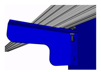
Mount additional trough brackets as needed. Most often, the middle leg and the back leg (farthest from the 0,0 home position) are used.
