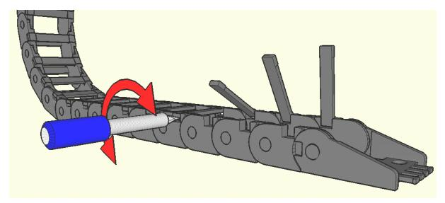
Insert the tip of a flathead screwdriver into either side of the hinged access bar. Turn the screwdriver approximately 1/4 turn in each direction until the sides of the access bars release. Open the access bars to run wiring that is common to the machine.
