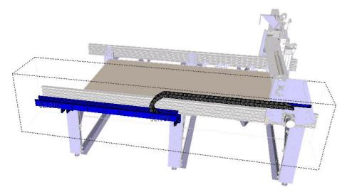
The above image shows how the E-chain installation looks on a 96" PRS.
