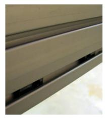
Install two T-nut ball & spring pivot inserts (000728) and on the inside face of the tableside in lowest slot.
