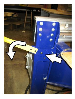
To unlock, pull the bar back towards you and lower them down. In this position, you will still be able to move each axis but the spindle will be deactivated.
