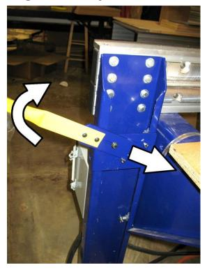
To lock bar into place: pull up from the vertical position and then slide the bar in towards the table. This locks it into place and activates the switch, allowing full operation of the machine.
