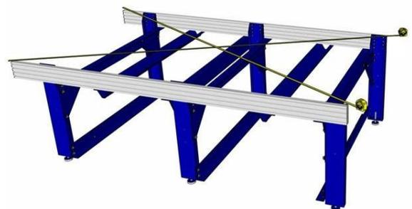
This example is exaggerated to illustrate the correct method of squaring the table:
