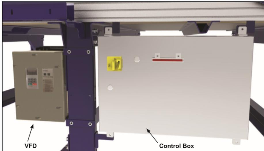
The **control box** is the “brain” of the machine and contains a control board, motor drivers, and other electronic components that allow the tool to move with precision, accuracy, and power. It connects to the computer through a single USB cable. The control box pictured here is for an alpha tool. Standard control boxes are smaller in size.
