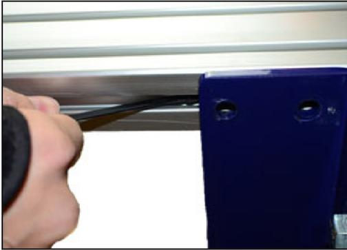
Use a zip tie to move the T-nuts (positioned earlier) so the threads are in line with the mounting holes.
