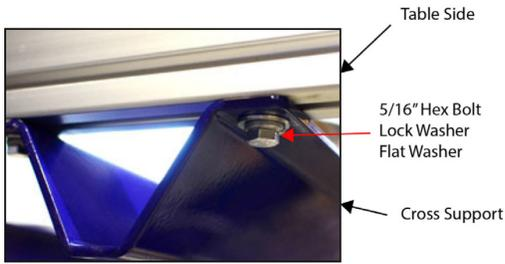
Attach each end of the cross support with 5/16" Hex bolt, Schnorr lock washer, and flat washer into the T-nuts.
