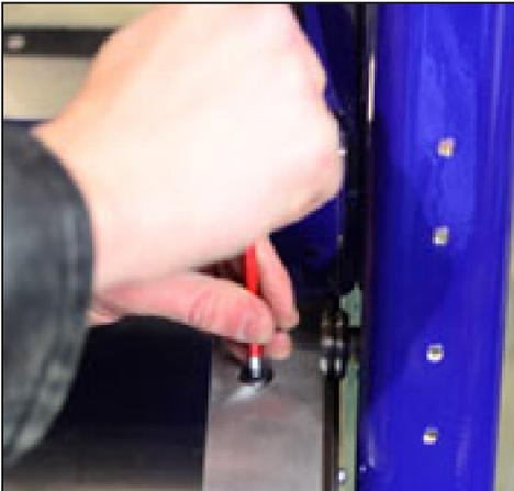
Align the rail by running the gantry up and down the length of the rail while watching from above to make sure rail is centered in the wheel. Starting at one end of the gantry, adjust, then tighten the rail as the gantry is slid down the length.
