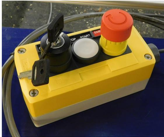
The second button on the pendant is a controlled stop button or “software stop” pressing this button will send a signal to the software to pause the cut and turn off the spindle. This stop will take longer to execute than an emergency stop but the accurate position of the tool will be maintained.
