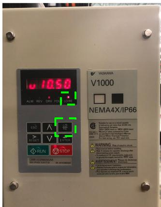
Next, check the settings on the VFD. Locate the button labelled “LO/RE” and press it. A red led should light up next to the LO/RE indicator below the VFD display. This will allow you to control the spindle from the VFD control pad. Press the green “RUN” button to start the spindle. Press the red “STOP” button to stop the spindle. Once you are done with this test, press the “LO/RE” button again to turn off the indicator light.
