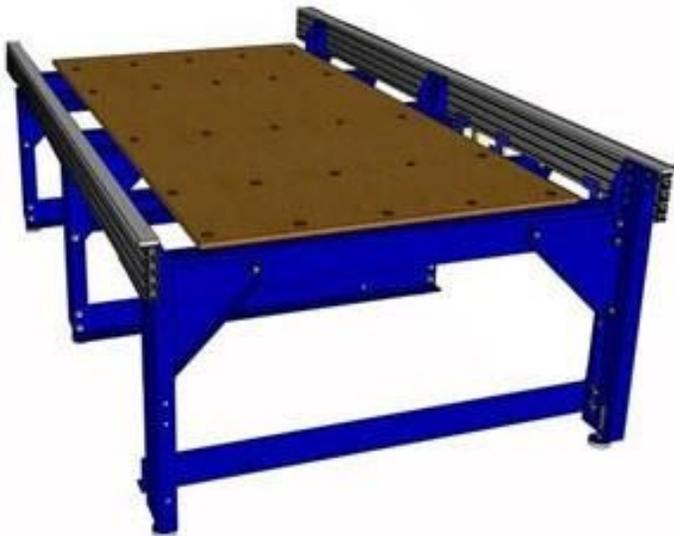
Use a 1" Forstner or spade bit to drill a counter bore deep enough for the head of the carriage bolt to sit below the surface of the plywood.
