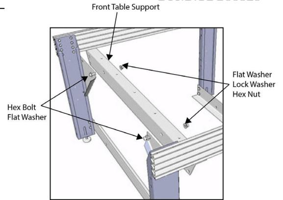
The middle legs will have upper table supports on both sides of the leg, but only one side uses gussets.
