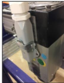
Arch spindle cable over the YZ car and connect to the spindle, locking connector in place.
