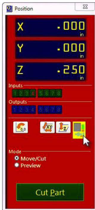
This panel provides essential machine information and controls. The following steps will walk through some of the most frequently used controls, including installing a bit, zeroing the machine’s three axes, and cutting a couple of sample projects.
