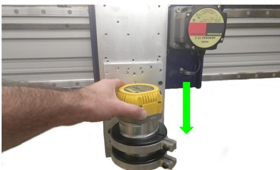
Lower the router all the way down into place, and tighten the two bolts in the mounting rings until the router is snug. It's important to make sure the bolts are tight enough to prevent twisting of the router while cutting.
