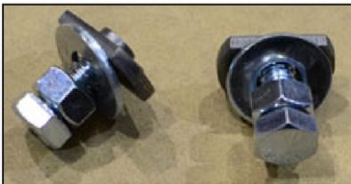
Assemble the X proximity switch targets with the 1/4-20x3/8 Socket Head Set Screw, T-nut, and 5/16-18x3/4 Hex Cap Screw.
