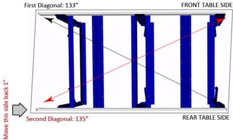
The rear table side should be moved half the difference between the two diagonal measurements. In the above example, there is a 2" difference between the measurements, so the rear table side should be moved 1". With one person holding the opposite diagonal in place, use a rubber mallet (or a hammer and protective block of wood) to carefully knock the table into square.
