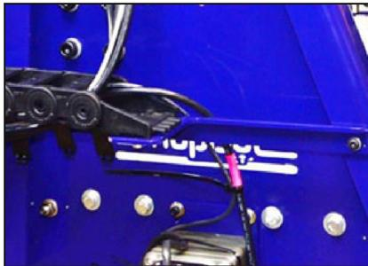
Connect the X-axis proximity switch cable (marked with red tape) by threading the nut onto the connector on the back of the switch.
