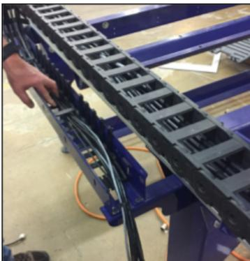
Loosely secure wire bundle to strain relief at bottom of cable carrier on same side as top.
