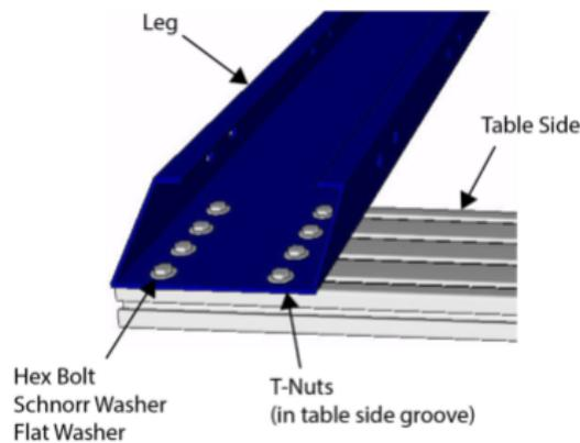
**Note:** Schnorr washers are concave washers. Install them with curve cradling the bolt head. Note that they can make threading the bolts into the T-nuts difficult. If necessary, use a zip tie or other shim behind the T-nut to force it closer to the surface of the slot so it is easier to catch the threads with the bolt assembly.
