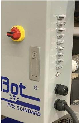
On the outside of the box, above the cord grips, you will find a series of labelled WAGO connectors. These provide connection points for your motors, control pendant, limit switches, z zero plate, spindle logic cable and USB communication cable.
