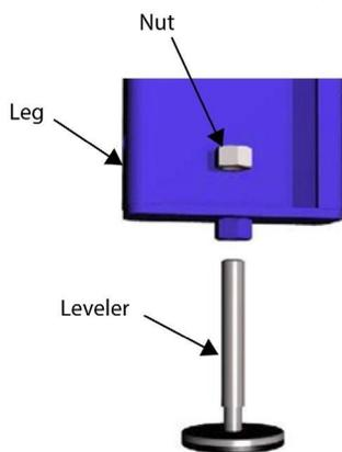
Remove table legs from packaging. Screw leveler approximately half way into the bottom of each table leg. Thread a 5/8" hex nut onto the leg leveler. Keep nut loose until table is leveled.
