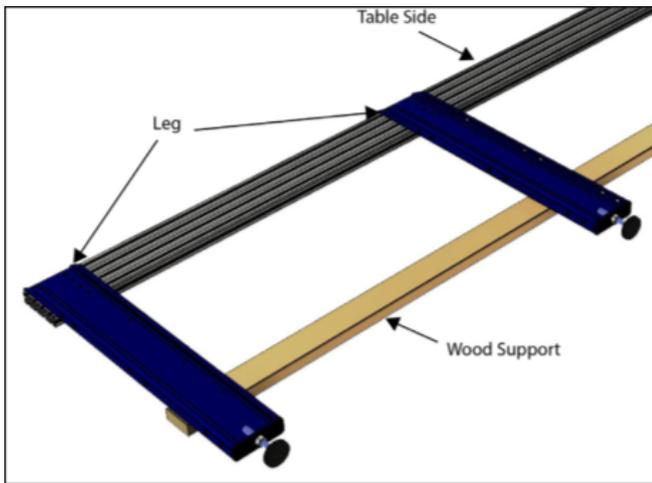
With the T-nuts in place, position the table legs to line up with them. Support the table legs so they stay level during installation.
