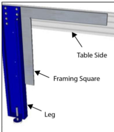
Hold a framing square against the leg and the table side while bolts are tightened to ensure leg is installed at a 90° angle. **Hand-tighten the top and bottom bolts** when the leg is square. **Do not tighten other bolts at this time.**
