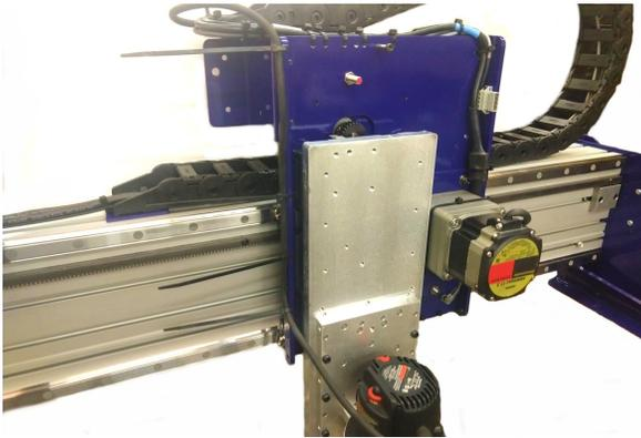
Using zip ties, run the power cable from the router up the left side of the blue Y carriage plate, and then into the echain. Make sure there is enough slack in the cable so it doesn't bind up while the Z moves up and down.
