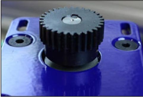
Slide pinion onto motor shaft while ensuring the key stays in place. If resistance is encountered, loosen set screws with 1/8" hex key.
