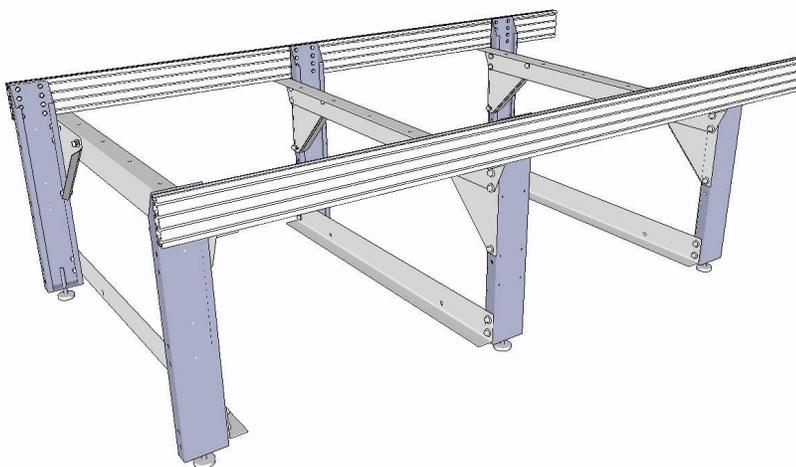
Install the remaining gussets and table supports using 1/2" hex bolt and flat washer on one side, and flat washer/lock washer/hex nut on other side.
