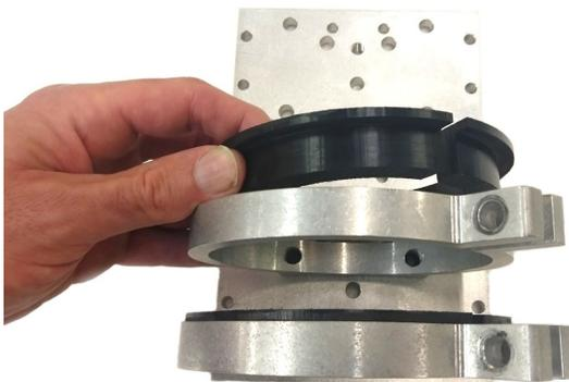
Insert the two black adapter rings (006229) into the two mounting rings on the mounting plate. Make sure the notches in the adapter rings line up with the notches in the mounting rings. You may need to loosen the two bolts located on the mounting rings to allow the adapter rings to drop in place.
