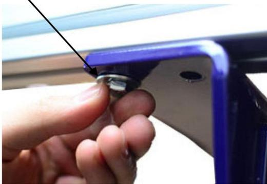
Attach the upper table support to table side with two 5/16" hex bolts, SCHNORR lock washers and flat washers on each side of the upper supports.
