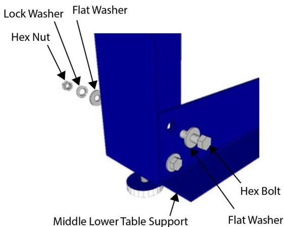
Secure middle lower table support to middle set of legs with the same order of 1/2" hex bolt and flat washer on one side, and flat washer/lock washer/ hex nut on the back side. Snug the bolts enough to preload the lock washers.
