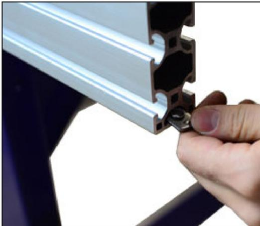
The upper table supports and cross supports are fastened to the table sides with threaded T-nuts. Insert T-nuts so the solid face is to the outside (face down) of the slot and move them to their approximate locations before mounting any components.
