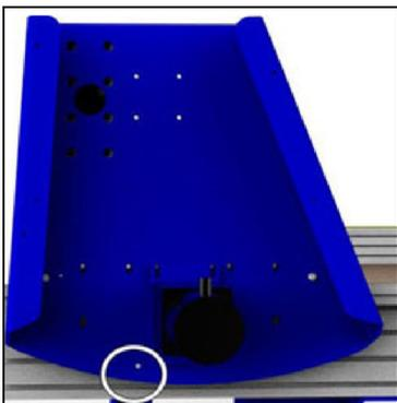
The X proximity switch is mounted in a threaded hole near the X1 motor on the gantry end plate.
