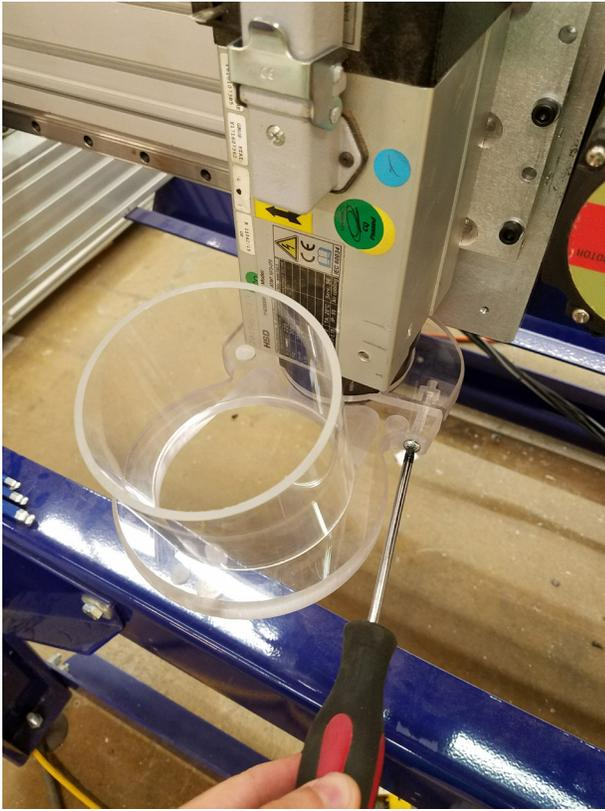
The mount for the dust shroud clamps around the collar of the spindle and can be tightened with a Phillips head screwdriver.
