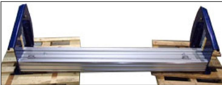
With help from another individual, remove gantry from packaging and carefully place on floor near table. Before proceeding, ensure front rails are already tightened.
