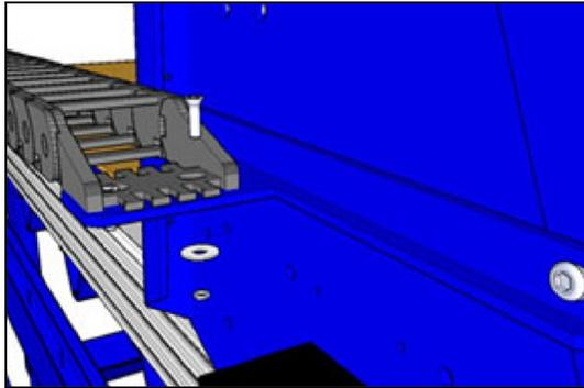
Attach one end of the cable carrier to the tab that extends from the X upper cable carrier bracket. Use flat head 10-32 screws, flat washer, lock washer and nut.
