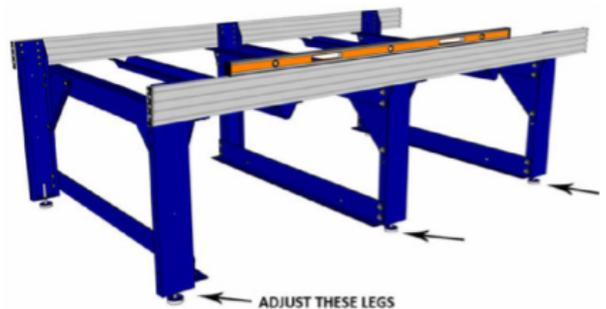
To adjust the other table side, place a long length of string around each corner so that they form an "X" in the middle of the table. Adjust the side of the table until the strings are very lightly touching. If the strings are overly tight or not touching, be sure to adjust **only** the one side, as the previous side should already be level.
