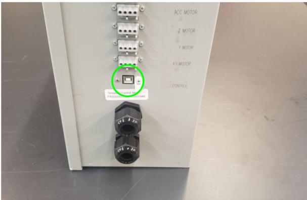
Plug the USB cable into the side of the control box and use a zip tie to secure the cable loop. The USB port is located just to the right of the cable entry port.
