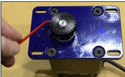
Remove any motors requiring pinion adjustment.
