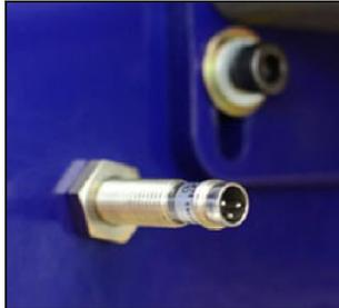
Rotate bolt so the three prongs are oriented as shown in the image at left. This ensures the cable will route cleanly.
