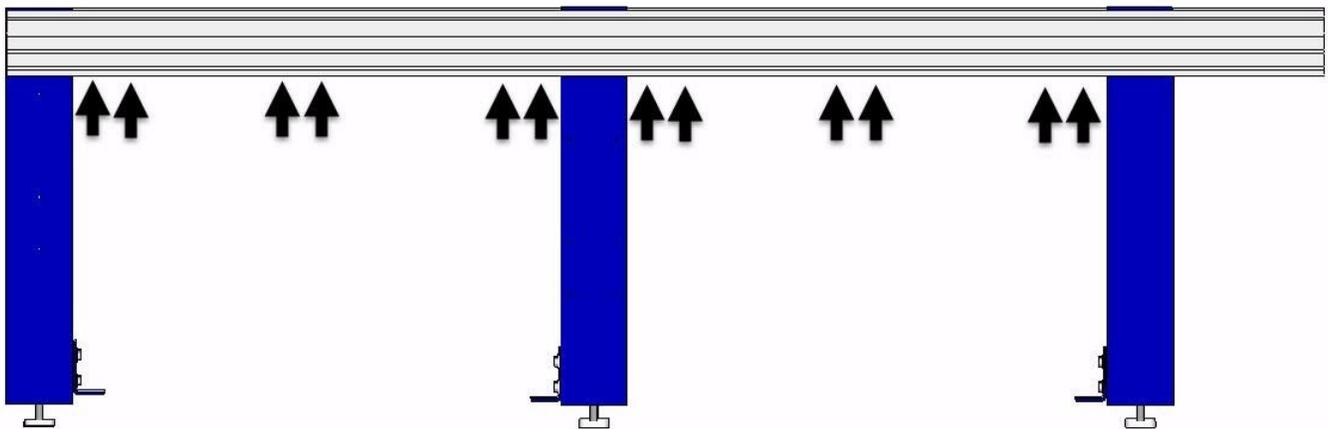
**Note:** This image shows the approximate T-nut locations for the upper table supports and cross supports for the PRS Gantry 96-48 table setup. A table configuration with more table legs or cross supports will require additional T-nuts as indicated on table drawing in the back of this guide. Two T-nuts are needed for every component.
