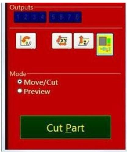
By default, the XY zeroing point will be the corner of the table nearest the control box. There is a program that will repeatedly and accurately find this point using the X and Y proximity switches. The XY zeroing program can be run by clicking on the “XY” button in the red position window. This is sometimes called a C3 routine, as entering C3 into the command line also runs this program.
