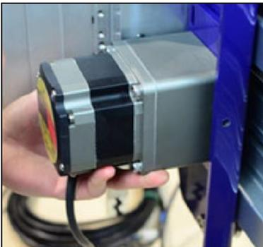
Mounting hardware (M6-1.0 x 12mm socket cap) is already fitted to the gantry end plates and YZ car where the motors will be mounted.
