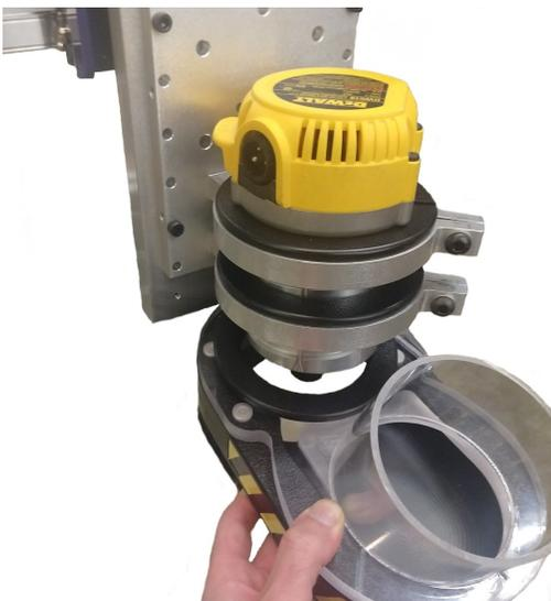
Loosen the screw on the side of the dust foot, and slide the dust foot with the adapter ring in place onto the router. It is a snug fit, so a little force may be needed. Tighten the screw on the side of the dust foot to clamp it in place.
