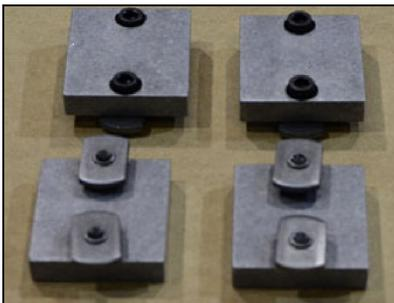
Assemble X-axis mechanical stop blocks using the X-axis mechanical stop, 1/4-20x1/2 Hex Cap Screws, and 1/4-20x3/8 Socket Head Set Screws.
