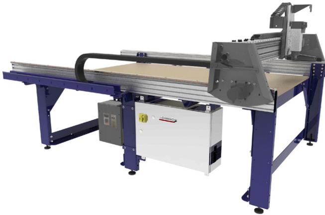
The base of the machine is referred to as the **table frame**.
