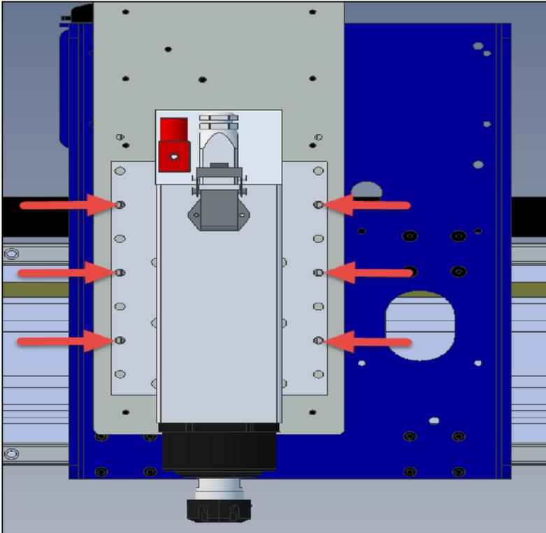
Using the six socket cap screws provided, mount the spindle to the Z-axis extrusion on the YZ car. If you experience resistance with any of the screws, uninstall and ensure the spindle is properly lined up with the holes before screwing in again.
