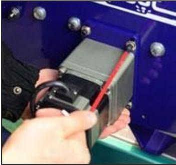
Push motor up to engage pinion with the rack. It may be necessary to slightly jiggle the motor to ensure teeth interlock.
