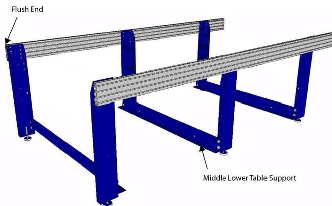
Install the middle lower table support. The horizontal flange should point to the front/flush end of the side rails.
