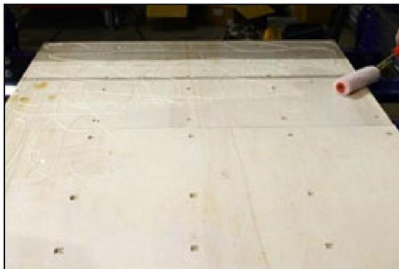
The spoilboard is a sacrificial layer of 3/4" Medium-Density Fiberboard (MDF). As it gets damaged over time, it can be re-surfaced to a perfectly flat work surface until the entire board has been used up, and then simply replace it with a new sheet.
