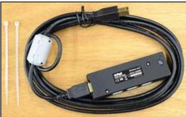
**Note:** The black box pictured at left is a USB hub. It prevents older operating systems from spontaneously reducing the USB communication rate. Use only the ShopBot communication cord with this hub.
