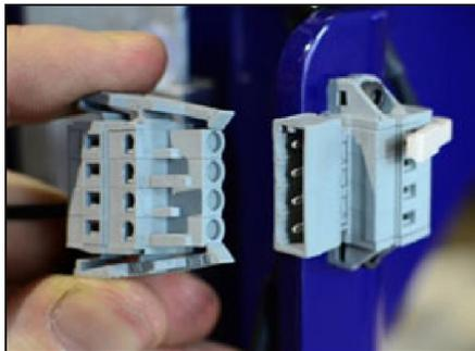
Insert the Z zero plate assembly Wago plug into the connector.
