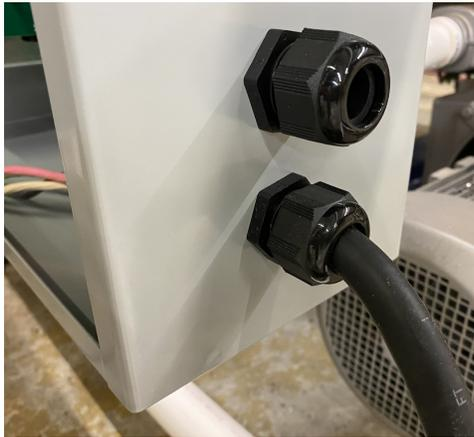
The spindle drive power cable will be connected to the output of the contactor inside the control box. Single phase systems will have a 3 conductor cable and Three phase systems will have a 4 conductor cable.
