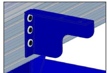
Repeat this step with the remaining bracket(s) (extended tables may have 3-4 brackets). Keep the mounting hardware loose so the brackets can slide along the table side in order to be moved into the proper position.
