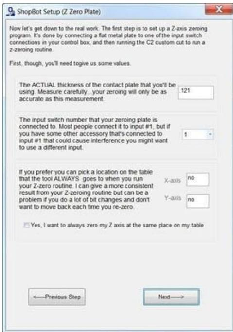
Zeroing the Z-axis is performed by placing the Z Zero plate on the zeroing surface under the bit and attaching the clip to the bit or collet. When the bit touches the plate a simple circuit is created, telling the tool to stop and record the location. This action is done using the Z zeroing program which can be run using the “Z” button in the red position window.
