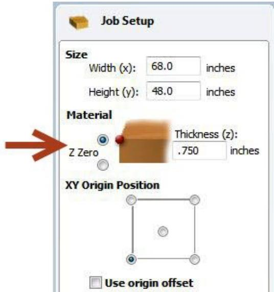
Zeroing to the top of the material is a better choice when a precise cut depth is needed (when cutting an inlay pocket, for example).
