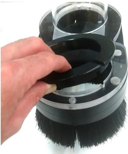
Grab the adapter ring (006266) with the two indents in the bottom, and place it inside the open ring in the dust foot.
