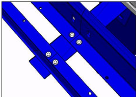
For models that need extended lengths of trough (longer than 96" in the X), use the second set of holes in the cable carrier bracket to install the troughs next to each other.
