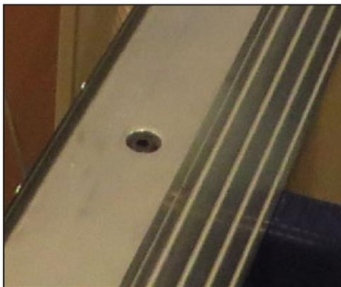
Place one 5/16" x 3/4" Button head screw into each counterbored hole in the top of each rail.
