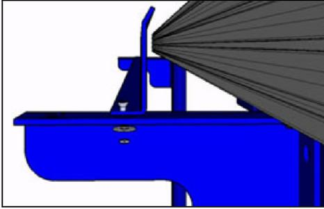
Position the first cable carrier trough so the holes closest to the edges are over the inside holes in the trough brackets.
