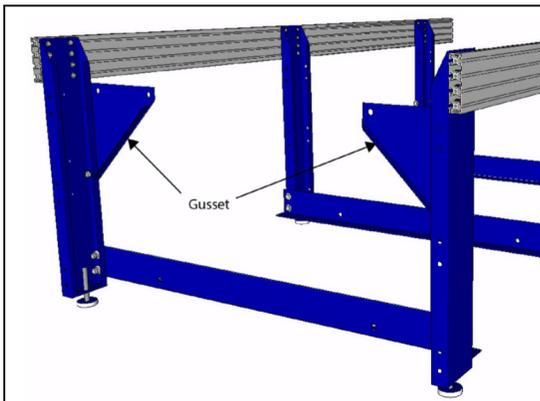
Orient the gusset with the flange facing the table leg. Use 1/2" hex bolt and flat washer on one side—flat washer, lock washer, and hex nut on the back side to secure the **bottom** corner of each gusset. When a gusset is properly oriented, the gusset flange will rest against the table leg, holding it in position. **Tighten bottom bolt only**; do not tighten the top bolt at this time.
