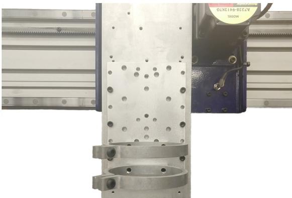
Start by mounting the router plate to the Z using the six M6-1.0 x 25mm SHCS (002925) that were provided with the tool. You can adjust the mounting plate up or down as needed for clearance depending on what you are routing.
