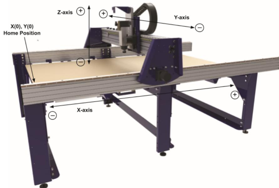
In most cases, the **X-, Y-, and Z-axes** will be referred to in respect to the machine. The **XY Home Position** is also indicated here.
