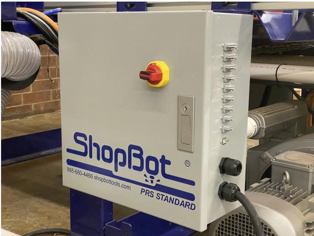
After the electrician has hooked up the PRS Standard Control Box, you can open the box by pushing in on the flip-out handle under the keyhole. The handle will rotate outward, providing a place to grab and pull the control box door open.
