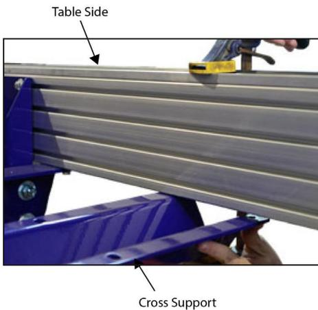
Use an assistant, clamp(s), or sling(s) to hold the cross supports against the bottom of the table side for installation.
