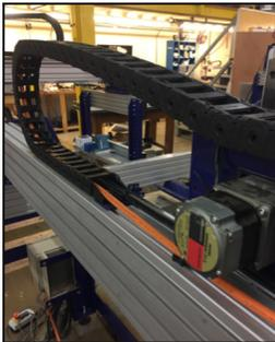
Run spindle cable up to Y cable carrier, following the path of the motor/proximity cable bundle. Open cable carrier cover and feed cable along opposite side of motor/proximity cable bundle. Close cable carrier cover.
