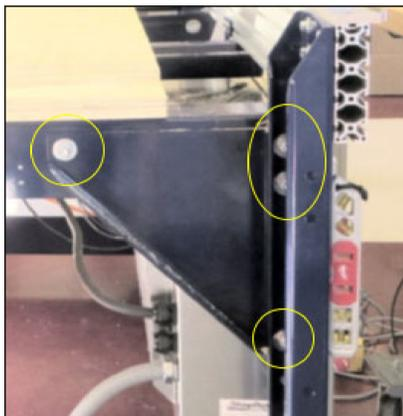
It is very important that the table is **level** and **square**. This means that all sides of the tool are on an even plane, and that the dimensions of the table are suitable to allow proper travel on all axes. Prior to leveling and squaring the table, ensure that it is located in the position where it will be used, as moving it can change these values.
