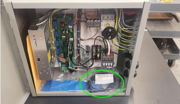
The USB cable is located in a packet inside the control box door.
