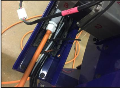
Uncoil spindle and run power cable from VFD under table to X cable carrier Open cable carrier covers using flat head screwdriver method from section 4 of this guide and place spindle cable into cable carrier opposite motor/ proximity cable bundle. Close cable carrier covers.
