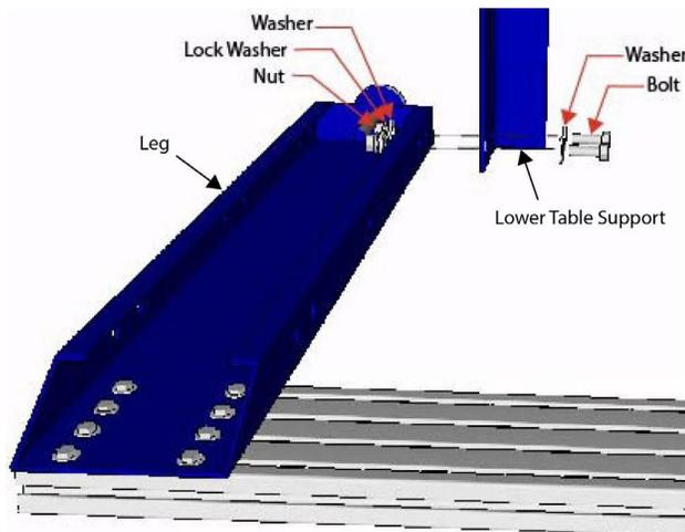
Install lower table support to the first exterior table leg with the L shape facing the interior of the machine with 1/2” bolt and flat washer on one side, and flat washer, lock washer, and nut on the back side. Tighten the bolts only until they are snug; do not tighten them completely at this time.
