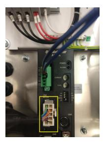
To complete the wiring, connect the accessory motor cable with the yellow band that was routed through the cord fixture to the white plug on the face of the newly installed driver. This completes the wiring portion of the indexer installation.
