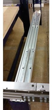
After the carriage bolts are in place, adjust the beam left-right so that it is an equal distance from the hanging bracket on either end. There should be about a  $\frac{1}{2}$  gap.
