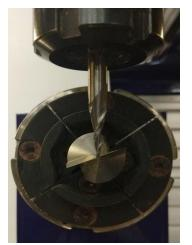
Center the spindle, as close as possible, relative to the headstock. Once in place, use the fixed mode on the keypad to make fine adjustments.
