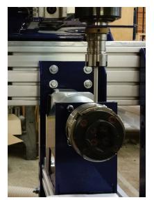
Use the same technique to align the indexer vertically, by bringing the drill rod down from above rather than from the side.
