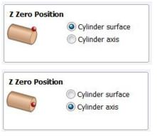
If zeroing Z to the surface, use the Z zero plate as usual.
