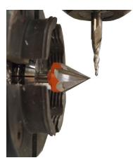
Chuck another fine bit into the spindle. Sharp ended bits allow precise identification of position relative to one another. Use the keypad to move the spindle bit about 1/8" in front of the center bit.
