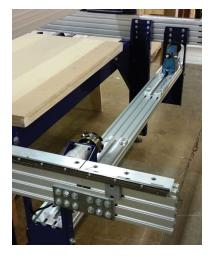
When mounting the headstock, push it laterally against one side of the aluminum t-slot plate to align it to the plate.
