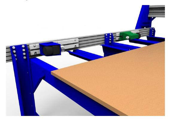
Using the hardware in the 6" indexer rail mounting hardware kit (included), attach the two T-rail base plates to one of your table sides. Use a level or straightedge to align the base plates with each other. Shown above is a 96"x60" PRS Gantry tool with a 96"x48" table surface. Leaving this extra clearance space around the indexer is not required, but it does allow the turning or larger stock.
