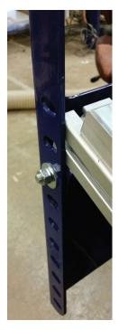
Attach the cross beam using carriage bolts, washers and nuts. For the 6" indexer, the 3rd slot from the top is typically ideal; for the 12", the 7th slot from the top. DO NOT TIGHTEN BOLTS - just thread them by hand.
