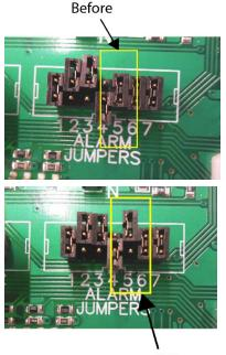
There are a set of alarm jumpers found on the right-middle of the control board. Remove the jumper on the one labelled "5" and install it so it is only attached to the top pin.
