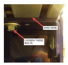
For very precise vertical alignment, shims can be inserted on the underside of the beam.
