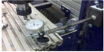
The first three setups are directly aimed at the pinion/rack adjustment. The last two, which will show lateral deflection at the bit, can show play in the lower YZ-car bearings, play in the Z bearings, or a loose spindle mount. To gain an accurate assessment at the bit, all play must be removed in the first three tests prior to setting up for the last two.
