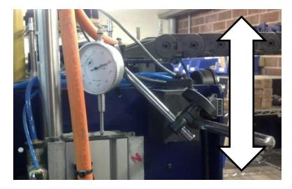
The following two setups have the base attached to a table leg and the indicator is touching a  $\frac{1}{2}$ " drill rod to measure deflection at the bit in the X and Y directions. Push/pull on the bit or collet nut directly at and away from the indicator.
