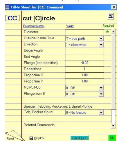
Passing the mouse cursor over the Parameter Name will display a 'Tool Tip' that explains the parameter. Passing the cursor over the value box will display the default setting for the parameter and it's range.
