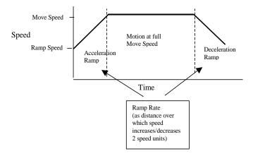
After the start of a move, speed increases during the ramp period from Ramp Speed (the starting speed) to Move Speed for the axis. Motion continues at Move Speed. Then at the end of the move, during the deceleration ramp period, speed decreases from Move Speed to Ramp Speed at which point motion stops. ShopBot's ramps are linear accelerations and decelerations. That makes the overall speed profile of a move a symmetrical trapezoid in time.
