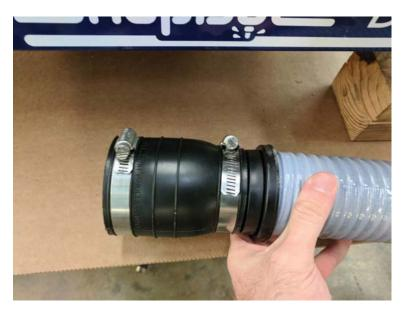
Route the hose with the rubber coupler under the machine from the rear. Place the rubber coupler over the PVC pipe and tighten in place with a flathead screwdriver.
