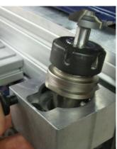
Place the loaded tool holders into the desired clip locations. Do not put one into the spindle at this time. Make sure the bits are facing **down**.
