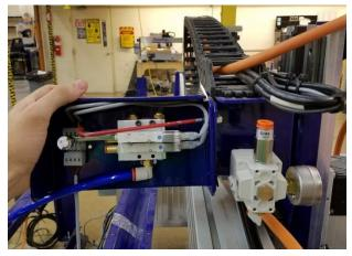
Using a 4mm hex wrench and adjustable wrench, connect the ATC manifold to the Y-Echain Bracket on the rear of the YZ car using the pair of pre-mounted hardware as shown above.
