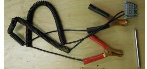
The red calibration clip will be clipped to the bottom of an empty tool holder as it is moved through all of the clip positions.
