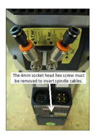
Plug the cables into the mating plug of the HSD spindle, taking note of the orientation of the cable plugs and being careful not to bend any of the pins. Insert the plug firmly into the socket and secure the socket head screw to lock the plug in place. Route the cabling from the spindle through the Yaxis E-chain into the control box and over to the left side of the ATC interface board.
