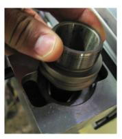
Press and hold the button on the side of the tool chuck. Rotate the tool holder until it seats into the chuck. Release the button to lock it into place.
