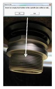
Place a second, empty tool holder, inverted in clip position #1.
