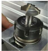
Tighten the collet nut to 100 ft/lbs with the ER32 spanner wrench. Do not over-tighten.
