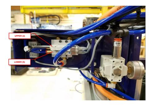
Turn on the pneumatics switch at the filter regulator manifold (near control box mounted to the table side) and verify that the pressure there is between 90 and 100 psi. Using too long of an air hose or an air hose of a small diameter can cause a lower pressure at the tool than what the main compressor tank is capable of. Using at least a 3/8" diameter air hose that is a maximum of 50' in length is recommended.
