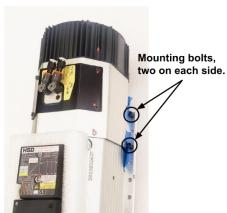
The ShopBot ATC is equipped with a 5HP fan cooled HSD spindle. An ATC system requires a minimum of 7 scfm at 90 psi of clean, dry, un-oiled compressed air which will be internally regulated to the following pressures:
