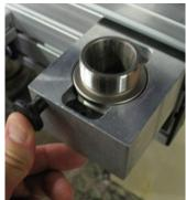
Snap the collet into the collet nut and thread the assembly onto the tool holder. Ensure the collet is the correct size for the bit needed.
