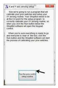
The next screen is "X and Y axis zeroing setup". Read this screen and click "Run the prox switch setup routine".
