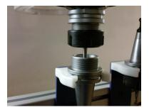
**Note:** This should only be a move in the Z-axis so that the tip of the drill rod is below the top edge of inverted clip. Do not move X or Y axes.
