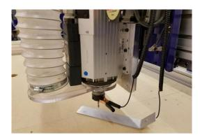
Note that the Z offset is reset to the Z home position any time the C3 routine is run. To permanently change the Z home position, refer to the Get plate offset (CN73) section of this document.
