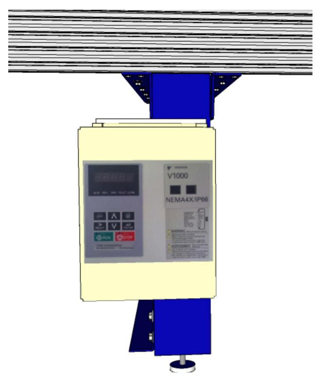
The 16" VFD will mount to the top and bottom set of holes in the middle leg of the ShopBot gantry tools with the VFD 1000 mounting kit (003065). If you have an earlier ShopBot that does not have 6 mounting holes on the front middle, it may be necessary to check the attached leg drawing in the appendixes and drill the upper and lower set.
