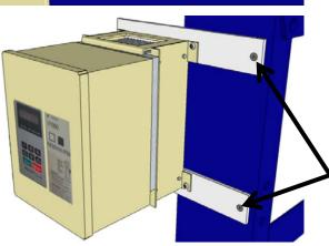
Use the 1/4-20x3/4 flat head screw in the last hole of the strap and fasten it securely to the leg with the 1/4" flat washer and 1/4" nylock nut. Repeat for both straps.
