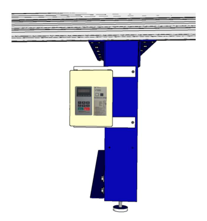
The 10" VFD will mount to the top and middle set of holes in the middle leg of the ShopBot gantry tools with the VFD 1000 mounting kit (003065). If you have an earlier ShopBot that does not have 6 mounting holes on the front middle leg, it may be necessary to check the attached leg drawing in the appendixes and drill the upper and middle set.
