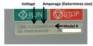
An example model number is shown to the left. The model number is CIMR–VU**2**A00**40**GAA.
