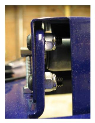
Close up view of screws that are used to fasten roller bar
