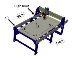
The X0 target is installed on the back left of your table.
