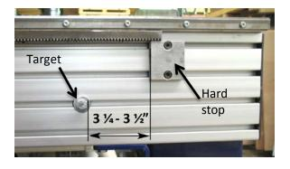
Slide one of the T-nuts into the lower-middle groove of the extrusion and lightly install a bolt and washer into it. Adjust the bolt until it is spaced about 3.5" from the hard stop.
