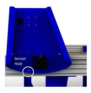
Check that the gantry can center the proximity sensor hole over the target without hitting the hard stop. The proximity switch hole is shown in the white circle to the left. Move the target as needed to achieve this and then tighten it. The goal here is to get the gantry close to the hard stop, but still have enough space to stop before hitting it. This will maximize your work area.
