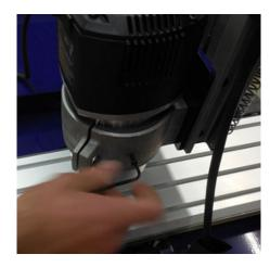
Loosen screw holding the router in place. Screw is protruding from the right side of the router mount.
