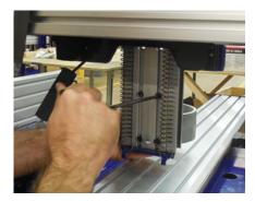
1. Install router mount to Z axis extrusion with four bolts.
