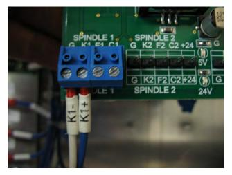
On the control board, remove the Blue wire (K1+) from its blue terminal block.
