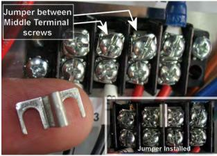
Using one of the Jumpers that were removed earlier, place 1 jumper on the top middle set of terminal screws.
