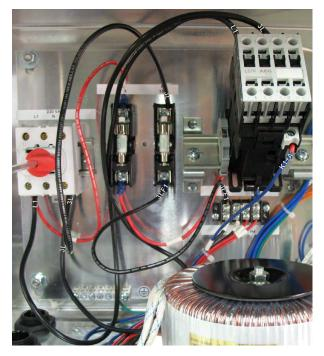
Take the loose end of the Black L1 wire from the contactor and wire into the main disconnect at position (2T1). This connection will be shared with a Red wire going to the top of the  $1^{st}$  fuse holder.
