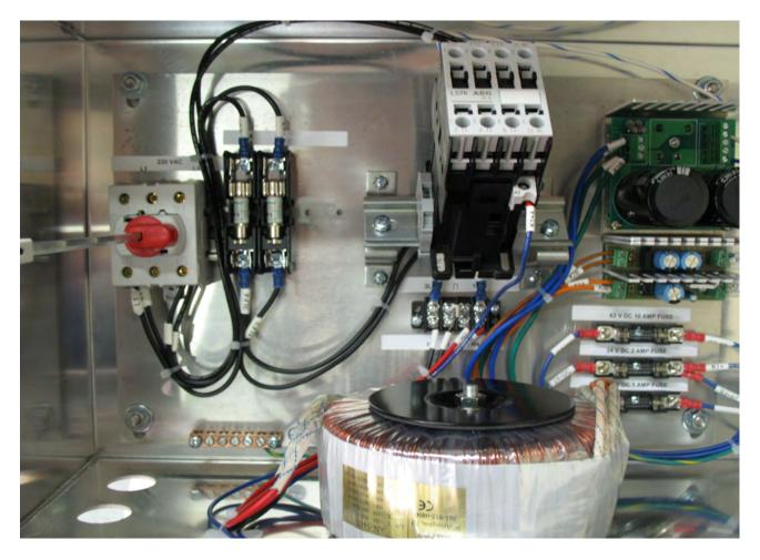
Overview - This document will walk you through the steps needed to change your 110 RBK Router control box over to a Spindle control box. We will be converting the power system from 110v (10270) to 220v single phase spindle (10272) or 220v three phase spindle (10273) depending on the spindle that you purchased. The ShopBot (15355) Router to Spindle Upgrade Kit for RBK control boxes is needed for this conversion.
