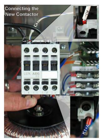
Locate the contactors and wires that came with the kit. The Blue/white wire (K1-) should be installed into the new contactor in position A1 located along the top and the Blue wire (K1+A) should be at position A2 on the bottom of new contactor.
