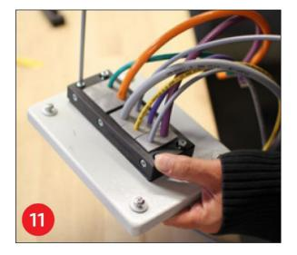
...and screw the cable entry frame to the control box.
