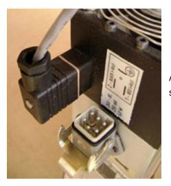
Attach the fan connection plug to the front face of the HSD spindle. Tighten the screw inside the fan connection plug.
