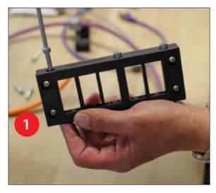
Loosen the screws of the frame.
