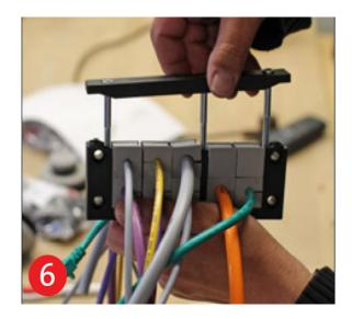
After completing the grommet placement set the cover strip on the frame again.
