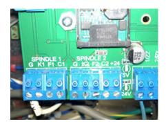
Connect the brown and white wires from the logic cable into the VFD terminals on the control board labeled "SPINDLE 1" (for a second spindle, use the terminals labeled "SPINDLE 2"). For Spindle #1, connect the brown wire to the "F1" terminal and the white wire to the "C1" terminal. For a second spindle, use the terminal connections" F2" and "C2".
