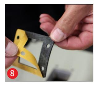
Remove the foil off the on-sided self-adhesive gasket that is included in the delivery.
