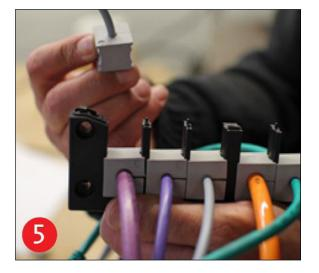
The flat side of the grommets in the upper row have to point downwards so that all flat sides rest on each other.
