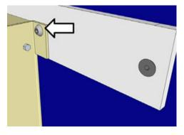
Use a 1/4-20x3/4" button head screw to attach the right upper hole of the VFD to the middle hole in the strap and upper left hole of the leg. Securely fasten the VFD and strap to the leg with 1/4" flat washer and 1/4" nylock nut. Repeat for the lower strap.
