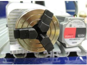
Chuck jaw configuration: gripping inwards
