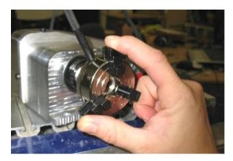
Once you have the jaws in the correct slots, maintain even pressure on each jaw while rotating the knurled ring clockwise. You don't need to apply much pressure, just enough to keep them aligned until the threads catch. Be sure that the jaws are moving evenly towards the center of the chuck. If they seem uneven, reverse direction and remove the jaws to start over.
