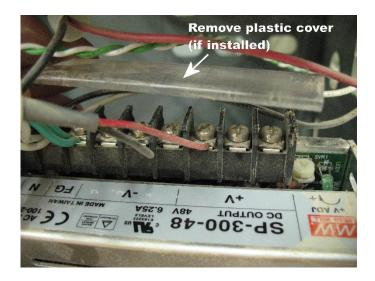
Wire the loose ends from the new 24v power supply into the 48v power supply. Be aware that there are pre-existing wires already in place. Black goes to L, White goes to N, and Green goes to FG. Tighten the terminals so that wires are securely fastened.
