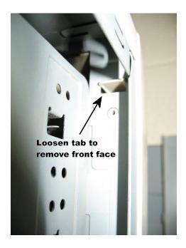
• Upon releasing the tabs from the main housing of the control box, slide the front face out of the way without disconnecting any of the wires that are still connected. Remove the two mounting screws that hold the power supply.
