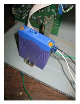
• Snap the 24v power supply to the mounted DIN rail.
