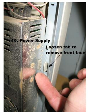
• Carefully swing the 48v power supply towards the open side of the control box and remove the plastic cover (if installed).
