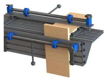
5. Finally, move the vertical board so that its top face is flush with the horizontal board. Make sure that both clamping mechanisms are tight before performing a cut.
