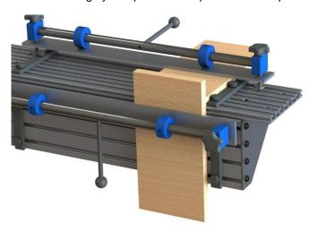
4. Position the vertical material so that both of its sides line up with the horizontal board's sides. Release the clamp to move it as needed. Once in position, slide the vertical fence up to the material and tighten it.
