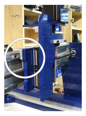
It will also be necessary to drill out the threaded holes in the side of the plate, shown here:
