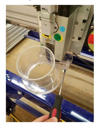
The mount for the dust shroud clamps around the collar of the spindle and can be tightened with a Phillips head screwdriver.
