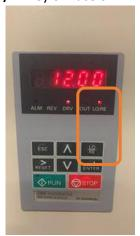
Pressing on the LO/RE button toggles the VFD to **LO**(cal) mode (light turns on.) In this mode, the operator must press on the Green RUN button on the face of the VFD to turn on the spindle.
