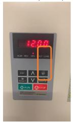
Normally, the VFD is in **RE**(mote) mode so that the software turns on the spindle when you are ready to run the file. In **RE** mode, there is no LO/RE light on the face of the VFD
