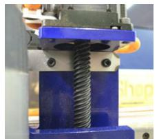
Reassemble the Z-axis. Prior to sliding the rail into the linear guide bearings, clean any sawdust or chips from the area to avoid pulling grit into the bearings.
