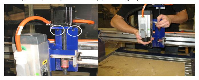
Carefully set down the Z-axis assembly. Remove two mounting bolts for the lead screw housing (photo below left), and four spindle mounting bolts from the back of the plate (photo below right). Remove the plate from the spindle.
