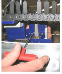
Remove six bolts and spindle from Z-axis. It may be necessary to move the Z-axis up and down to access all the bolts.
