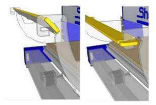
Slide the rear support bar (colored here for visibility) into the notches on the back of the side panels.
