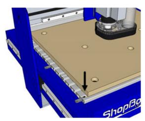
Slide one nut into the first slot on the table, then use the side panels as a guide for placement of the other nuts.
