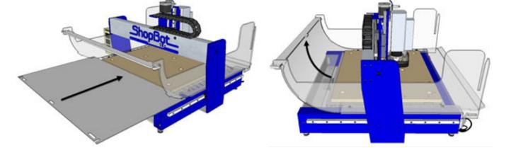
Slide the rear panel in from the back of the machine. Then wrap the back panel up and secure it to the tabs on the rear support bar.
