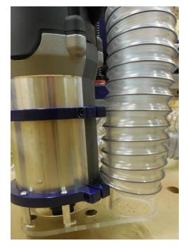
Move the router to the bottom of its Z travel, and install the hose so that it bypasses the first router mount and rests on the top of the second router mount as shown.
