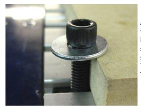
As with any ShopBot project, it is necessary to secure the workpiece before cutting. ShopBot recommends using the included T-nuts, washers, and 1¼" bolts. Center the 18x24" sheet on the table bed and position the bolts so they are snug against the sides. Tighten the bolts into the T-nuts. Test the hold-down strength by trying to move the board. There should be no movement.
