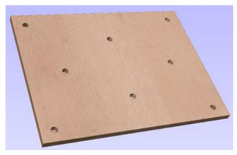
ShopBot has created a cut file with a drilling pattern for an 18x24" work surface. This will not cover the entire surface of the table bed; the ShopBot is capable of about 1" of over-travel to ensure that it can cut past the edge of parts.
