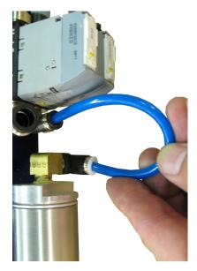
Use 1/4" tubing to connect the 1/4" push-in connectors.
