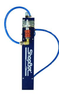
Connect the upper push-in of the dual valve to the 1/2" push-in of the air supply assembly using the length of 1/2" tubing that was originally removed from the SV air drill.
