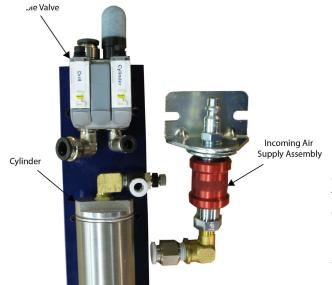
Slide out two mounting tabs from the back side of the double valve and position double valve on the cylinder side of the air drill.
