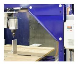
Use the keypad to move the spindle to the A/B home position (spindle straight down and B motor pointing to plus Y). Move as close as possible by eye. Do not rely on the coordinate readings in the red position window – they may not be accurate if this calibration routine is necessary. Move the drill rod over the top face of the block. The correct position is shown at left.
