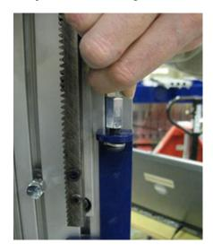
Pull the cylinder rod downward so that it aligns with the tab on the lower pneumatic assist bracket.
