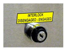
Locate the key attached to your collet wrench. This will be located either inside the control box, or in one of the hardware boxes. Insert key into safety lockout on the main control box, and turn key to "ENGAGED."
