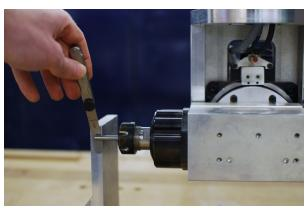
Move the spindle so the drill rod is lightly touching the front face of the block.
