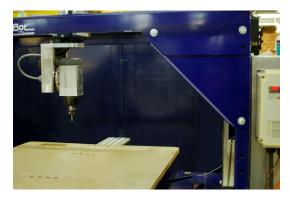
Use the keypad to move the spindle to its A/B home location shown at left.
