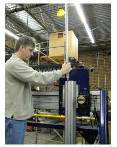
Remove the two 1/4-20 screws from the upper pneumatic assist bracket, and the 5/16-24 screw from the end of the cylinder rod. Mount the cylinder to the front of the YZ car on the left side of the Z-axis extrusion.
