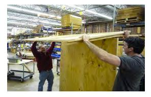
Remove the screws at the top edge of the crate and lift/ slide the top off. Unscrew edge brackets and freight gussets, and carefully remove crate sides.
