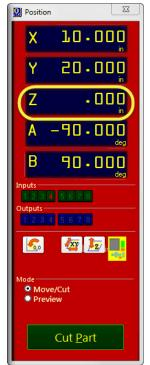
Once the rod is in position on top of the block, exit the keypad and type a **ZZ** command. Check the coordinate window to make sure that this command has been accepted.
