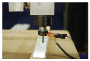
Plug in the Z-axis zeroing plate assembly and connect the grounding clip to the collet nut. Place the Z zero plate onto the material or the table base and click the Z zero button in the position window. This is a shortcut to the Z zero file (also known as C2).
