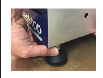
Use the levelling feet to level the tool on the workbench surface.
