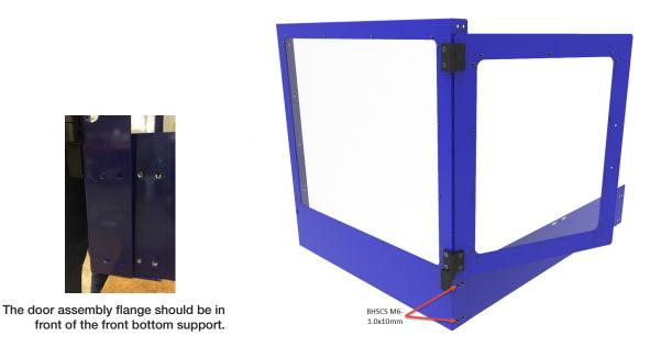
Lift the ShopBot Desktop tool to set the back feet on top of the Back Bottom Support flange. Attach the Back Bottom Support to the back side of the Left Door Assembly using 4 BHSCS M6-1.0x10mm. Do not tighten the bolts at this time.
