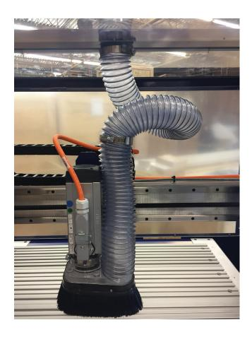
Clamp should be used to mount dust hose to top flange.
