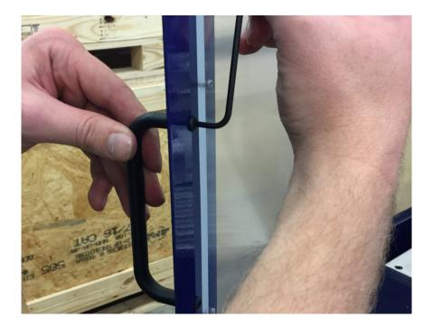
Attach the Top Support (the one with the magnets) to the front of the enclosure using 8 BHSCS M6-1.0x10mm, 4 on each side. Do not tighten the bolts at this time.
