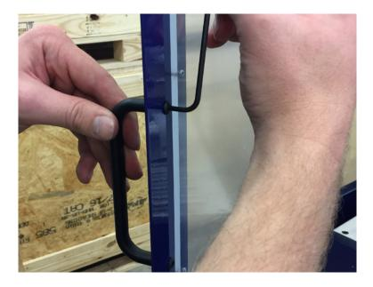
All plastic panels are installed from the inside of the enclosure, with the screws installed from the outside. The rear panel should be installed **first**, followed by the top back and the top front.
