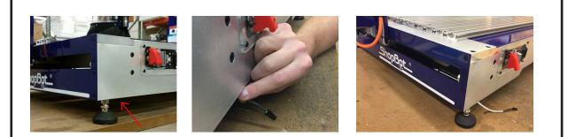
Locate the interlock connector on the right side of the tool. It will be under the tool near the red power switch. Leave it attached, but extend it so that it is laying to the side of the tool for accessibility during assembly.
