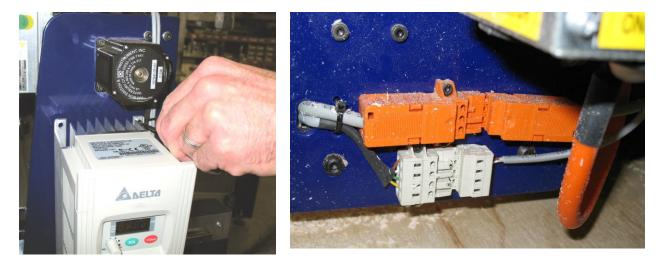
The two loose plugs coming from the bottom of the VFD need to be plugged in at this point. Connect each one to its matching plug on the gantry. Make sure that these connections are tight. Complete the installation by securing the spindle cable to gantry with a couple of zip ties (you may have to cut the old ones out first-just be careful not to cut any of the cables).
