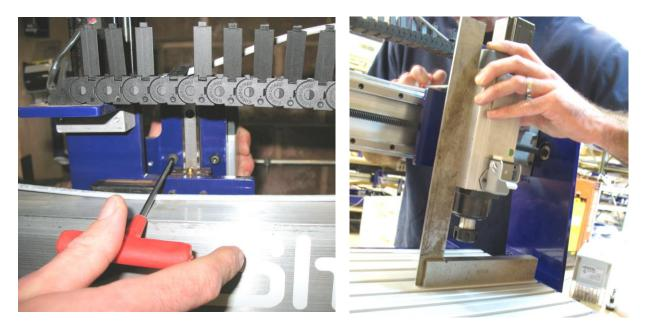
Bolting the spindle to the Z-axis
