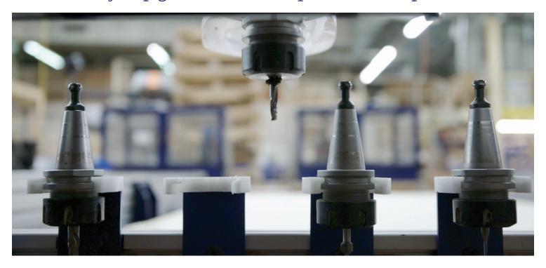
ShopBot's Automatic Tool Changer (ATC) is available on our full size PRSalpha Gantry CNC tools. It's powered by an HSD ES915 5hp spindle.
